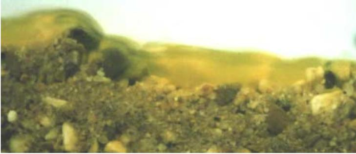
**Fig. 21.2.** Small-scale simulation of bed load transport in the laboratory. The solid and liquid phases are distinct (water was coloured with fluoresceine). The typical flow depth in these experiments was 1 cm
