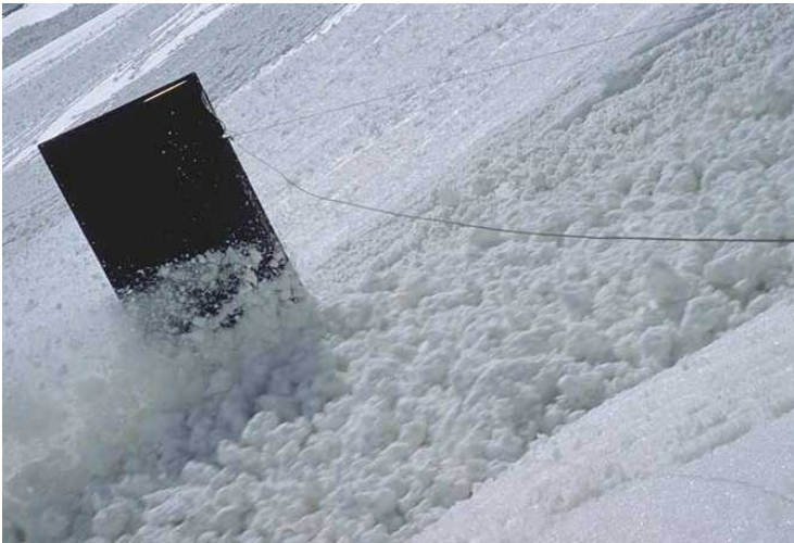
Fig. 13.2. Flowing avalanche impacting a wing-shaped structure in the Lauratet experimental site (France)
