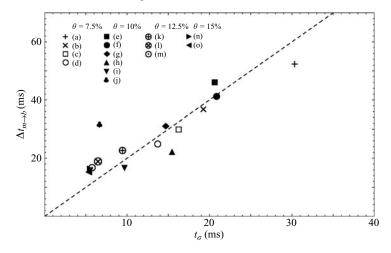
FIGURE 10. Comparison between the mean experimental lag time  $\Delta \bar{t}_{mb}$  and the theoretical value  $t_{\sigma} = 1/(\bar{N}\sigma)$ . The dashed line stands for the empirical trend  $\Delta \bar{t}_{mb} = 2t_{\sigma}$ .
