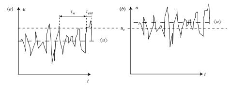
FIGURE 3. Fluctuations of the instantaneous velocity u around the mean value  $\langle u \rangle$ . (a) Mean fluid velocity below the critical threshold  $u_c$ . (b) Mean fluid velocity in excess of the critical threshold  $u_c$ . In both cases, particle entrainment occurs sporadically.
