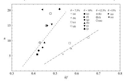
FIGURE 6. Variation in  $\dot{n}$  with  $\bar{u}_f$ . The dashed lines represent empirical trends adjusted on the data:  $\dot{n} = 90\bar{u}_f - 30$  (dashed line) for  $\tan\theta = 0.1 - 0.125$  and  $\dot{n} = 45\bar{u}_f - 18$  (long dashed line) for  $\tan\theta = 0.075$ .
