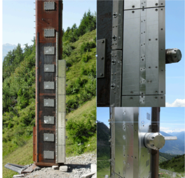
Fig. 1: The 20 m high tower is instrumented with high-frequency load cells, optical sensors for velocity measurements and flow depth sensors.
